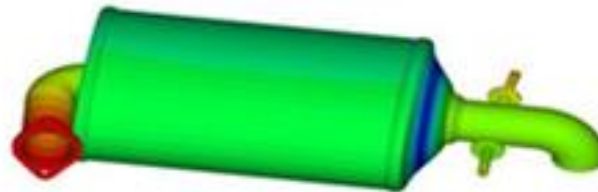
Fig 12: This page provides a comprehensive examination of the exhaust muffler. The thickness of the shield is 1 millimeter.
