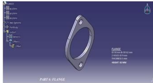
Fig 10: A piece of equipment known as a flange is utilized in the process of connecting two pipes or other types of equipment to one another.
